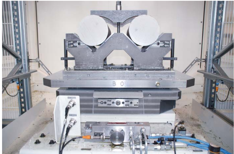
The example shows a mechanical jig. The exchangeable plate is equipped with a zero point mounting system SPEEDY classic 4
