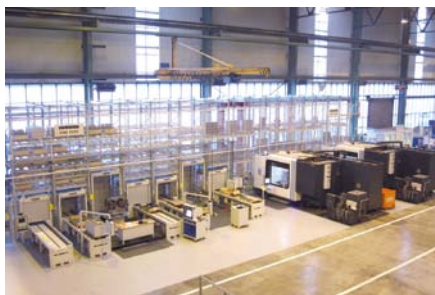
Pallet station with more than 50 jigs
