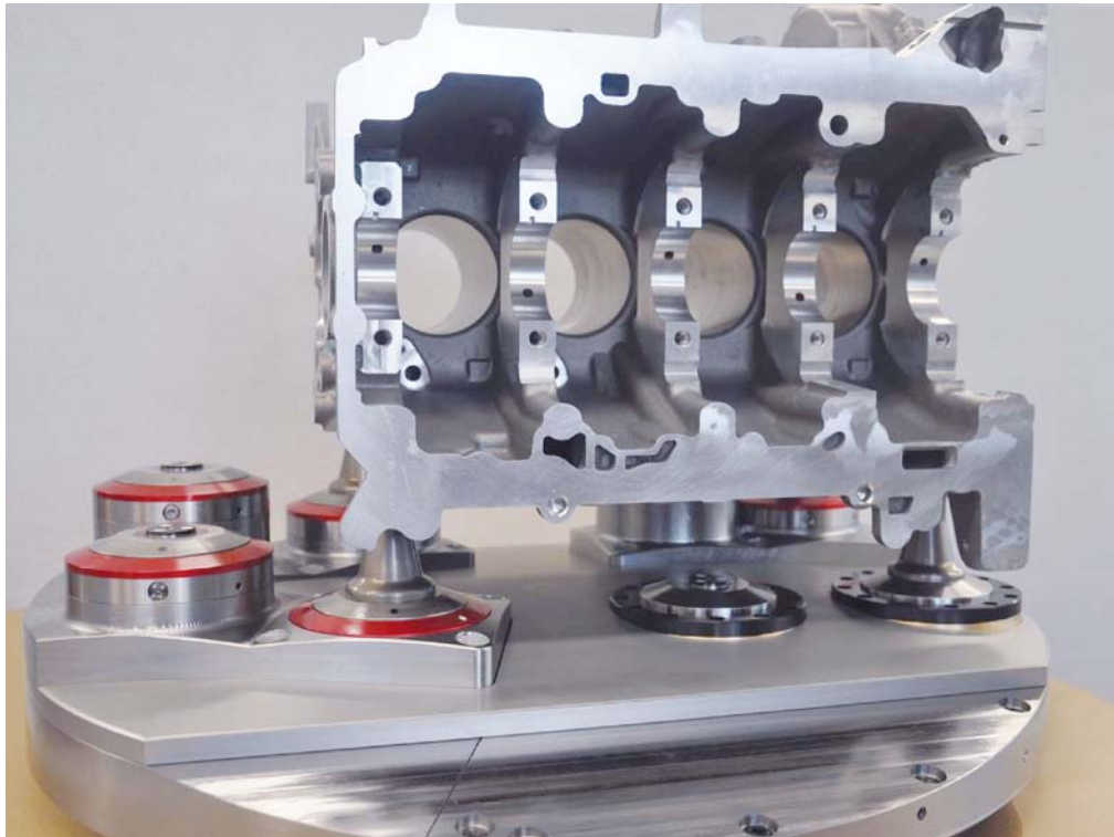
Workpiece with multiple clamping and support points
