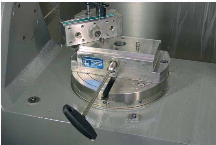
Fast clamping block with SPEEDY metec 2.
