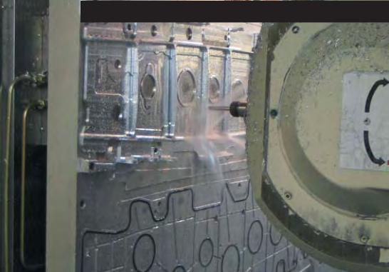
Left: One of three SNK HPS-120B machines tackles ribs on a vacuum fixture plate
